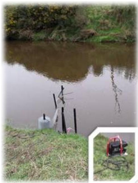
Figure 4: DIDSON set up at site downstream from the Top Falls (DIDSON in insert). The wire mesh directly downstream from the DIDSON ensures that kanakana swim within the operating field of view.
